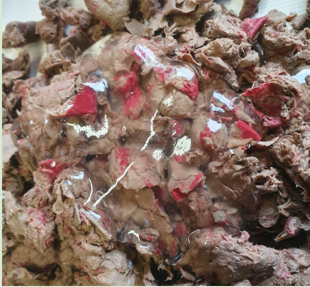
Cardboard pulp with wet mix over it, before mixing
